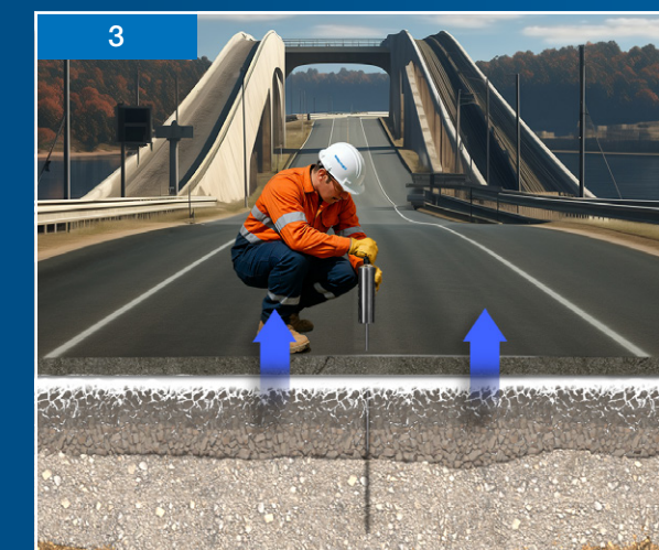
Continued injection raises, and re-supports the roading.
